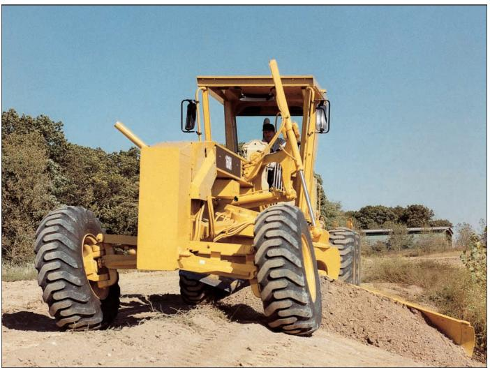
**Blade positioning.** The blade linkage design enhances moldboard positioning. This blade linkage is most beneficial in ditch cutting and cleaning.
