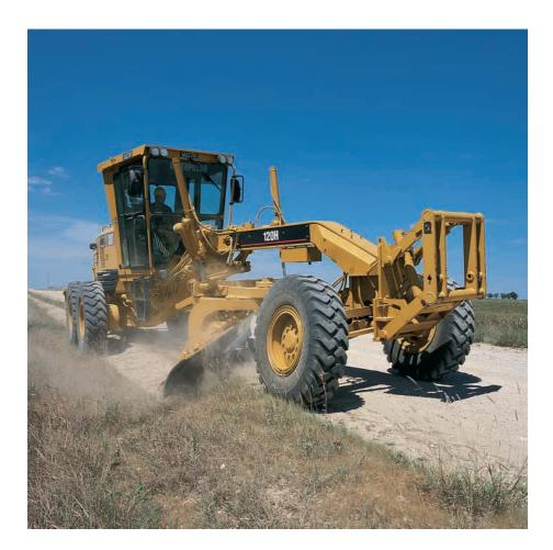
**Quiet Cab.** The resiliently mounted engine and transmission provide interior sound levels of 76dB(A) when measured with the doors and windows closed per ISO 6394. Lower interior noise levels improve operator working conditions. **Quiet Machine.** Exterior sound level of 107dB(A) when tested per ISO 6395, Annex B. The optional sound suppression group complies with the EU 2000/14/EC sound limit of 107 dB(A). This quiet operation lets the 120H work with minimal disturbance to the surroundings.
