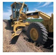
**Blade Positioning.** The blade linkage design provides extensive moldboard positioning, most beneficial in midrange bank sloping and in ditch cutting and cleaning.
