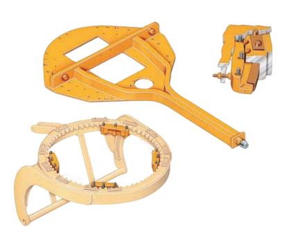
**Blade**. Heat treated moldboard rails, through-hardened, curved DH-2<sup>TM</sup> steel cutting edge and end bits, and replaceable metallic wear inserts assure a long, reliable service life. Three sideshift mounting locations for the optional moldboard add flexibility.
