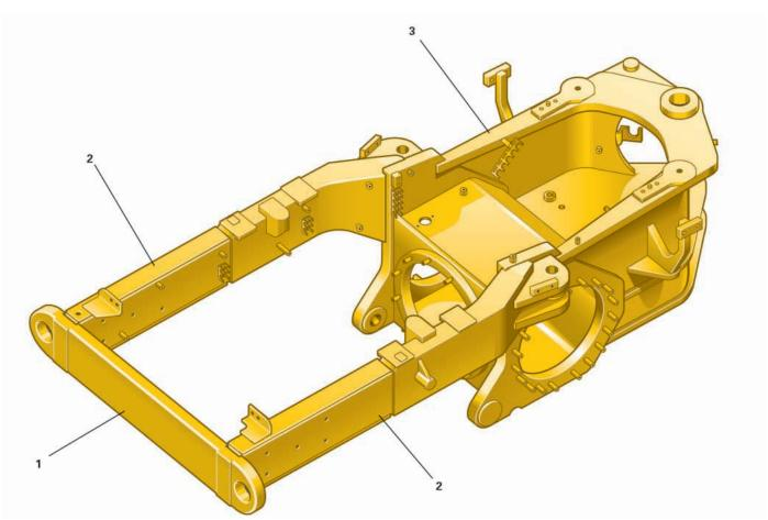
1 Integrated bumper; 2 Box-sectioned channels; 3 Fully welded differential
