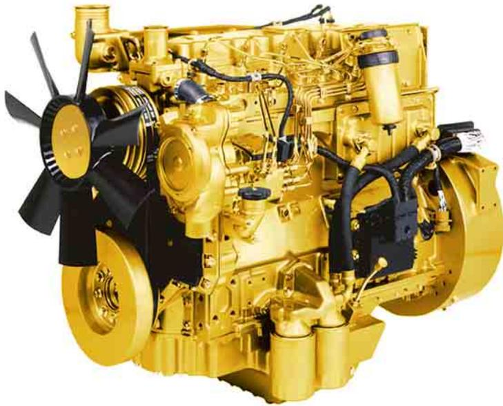
**Turbocharged air-to-air aftercooling.** It provides improved fuel economy by packing cooler, denser air into cylinders for more complete combustion of fuel and lower emissions.
