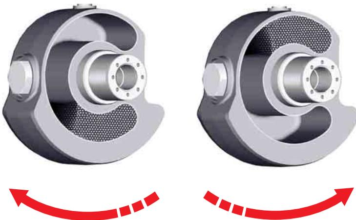
**Amplitude selection.** Positive amplitude selection is accomplished when the steel shot is repositioned inside the hollow eccentric weight. Direction of weight shaft rotation determines amplitude level.
