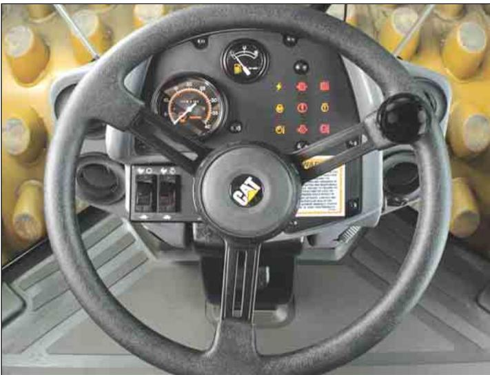
**Operational gauges.** Steering console and instrumentation gauges are infinitely adjustable within the tilt range to the desired position of the operator. Entire console tilts for simple entrance and exit.
