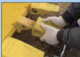
Set PAB tooth to horizontal pin type adapter
